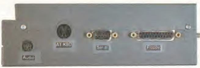
Connect a disk drive, a modem, an audio source and even a keyboard. The SX-1 uses an AT101-style keyboard rather than the standard A4000 unit.
